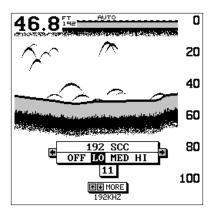
sensitivity of the receiver, decreasing it near the surface and gradually increasing it as the depth increases. The maximum depth that SCC will affect is 75% of the selected depth range. For example, on a 0-60 foot range with maximum SCC, surface clutter will be reduced down to 45 feet.
